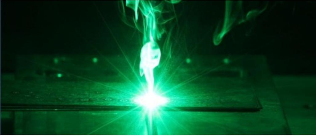
Using green light, copper welding becomes more energy efficient and of higher quality, irrespective of the properties of the material surface. © Oliver Graf
